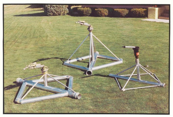
The Schumacher aluminum volume gun stands are rigid for high strength. They are designed so the base fills with water for weight and stability. The aluminum gun stands are so lightweight that when empty, one man can easily handle them for loading and unloading.
